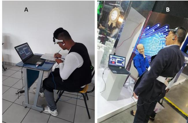
Fig. 3. A) Posture sensor placed in the vest. B) Posture sensor placed on the body band.
